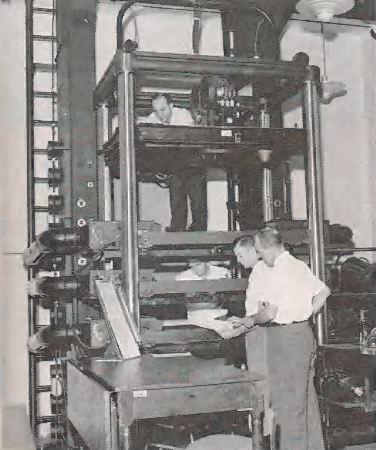
Production camera supervisor Dick Grills checks the multiplane camera set-up with operator Ed Cook, while assistants Paul Whitehouse and Jim Pickel adjust the different planes for the next shot on Disney's unique multi-plane camera system, which was invented by Ub Iwerks.
